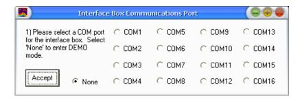
Be sure that the all deice is attached to your PC and that +12VDC power has been turned on. Select the COM port where the Echosounder is attached and click on "Accept". If you do not have a Echosounder attached (to run the software in demo mode and/or to playback some prerecorded files), select "None" and click on the "Accept" box.
